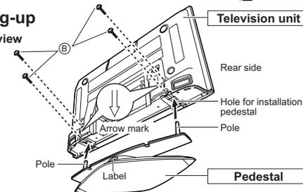
\* Place pedestal on a horizontal and level surface.
