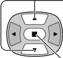
Press to select START TIME/ FINISH TIME (When TIME OF DAY is selected). Press to select SHOW DURATION/ SAVER DURATION (When INTERVAL is selected).
