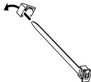
To secure cables connected to Terminals, wrap the cable fixing band around them then pass the pointed end through the locking block, as shown in the figure.
