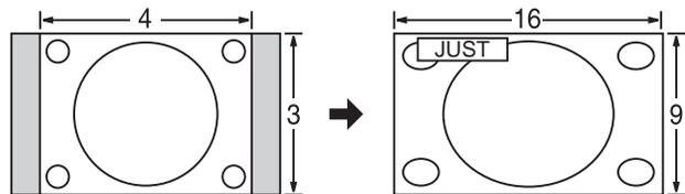
Stretches to justify the 4:3 image to the four corners of the screen.
