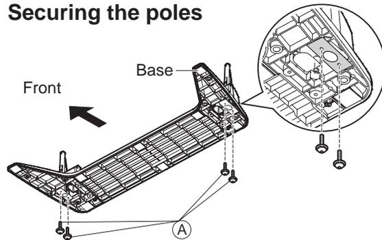
Use the assembly (A) screws to secure the poles firmly to the bottom of the base.
