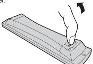
2. Install the batteries as shown in the battery compartment.
