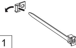
To secure cables connected to Terminals, wrap the cable fixing band around them then pass the pointed end through the locking block, as shown in the figure.
