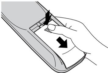
2. Install the batteries as shown in the battery compartment.
