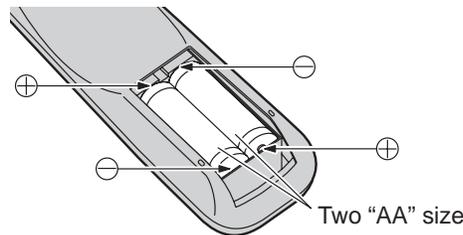
3. Replace the cover and slide in reverse until the lock snaps.
