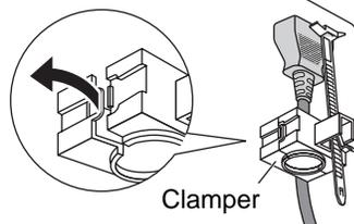
2. Insert the AC cord and close the clamper securely.
