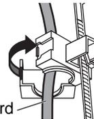
3. Slide up the clamper and fix the AC cord plug securely.
