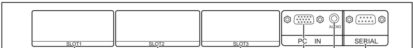
Optional Terminal Board Insert Slot (covered)
