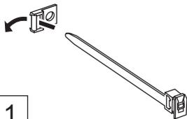
To secure cables connected to Terminals, wrap the cable fixing band around them then pass the pointed end through the locking block, as shown in the figure. **While ensuring there is sufficient slack in cables to minimize stress (especially in the power cord), firmly bind all cables with the supplied fixing band.**
