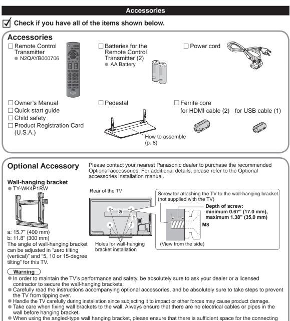
cables not to press against the wall when the TV is tilted forward.
