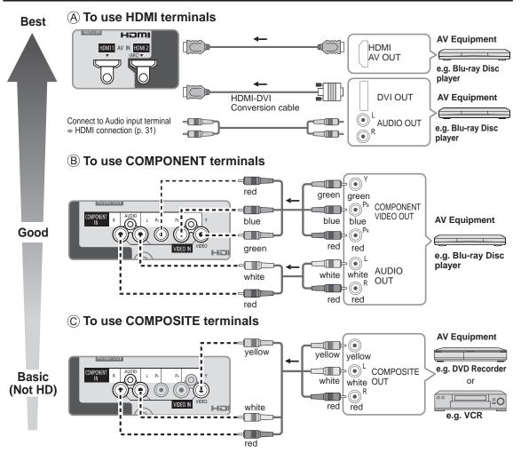
The Green terminal is shared for both the COMPONENT and COMPOSITE (VIDEO IN) connection. When using COMPOSITE (VIDEO IN) connection, the Yellow connector (Video) should be inserted into Green connection. (Watching content from external devices (p. 16))
