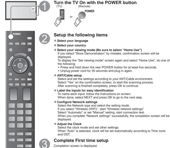
You can repeat the First time setup Press MENU -> Setup -> First time setup
