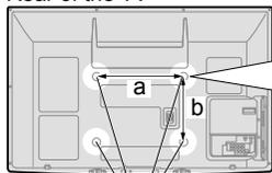
Holes for wall-hanging bracket installation
