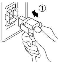
Insert it firmly until the tabs on both sides click into place.
