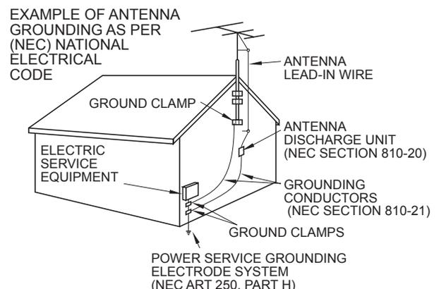
19) An outside antenna system should not be located in the vicinity of overhead power lines or other electric light or power circuits, or where it can fall into such power lines or circuits. When installing an outside antenna system extreme care should be taken to keep from touching such power lines or circuits as contact with them might be fatal.
