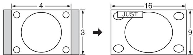
Stretches to justify the 4:3 image to the four corners of the screen. (Recommended for normal TV broadcast)
