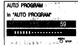
Channels will automatically advance until all channels have been scanned. Channel numbers with a video signal present will turn light blue. Which indicates it has been stored in the Channel Scan Memory.
