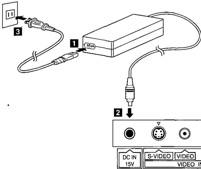
Connect the AC cable and power supply to the Wall outlet connecting the DC plug to DC in Jack
