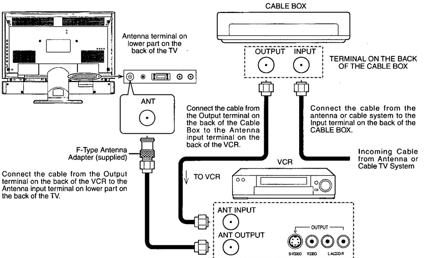
**Note:** When the antenna cable is connected to the TV antenna terminal via a cable box or VCR, set the TV channel to CH3 or CH4, cable. This does not apply when signal is input from VIDEO INPUT.
