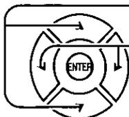
To reset to standard setting, select NORMALIZE with the up ▲ and down ▼ buttons and press ENTER. BASS, TREBLE, BALANCE and SURROUND adjustments are stored for each AUDIO menu.
