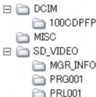
[DCIM]: The images (IMGA0001.JPG etc.) in this folder are recorded in the JPEG format. ([100-0001] or similar indication is displayed on the SD Video Camera.)
