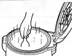
When not operating or taking the pan out of the body, be sure to push the "Keep Warm" button up and confirm the lamp goes OFF.
