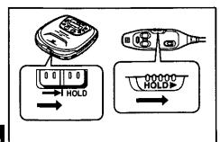
This function causes the unit to ignore short, accidental button presses. (The disc lid can still be opened and closed.)
