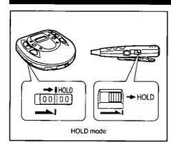
This function causes the unit to ignore accidental button presses. (The disc lid can still be opened and closed.)
