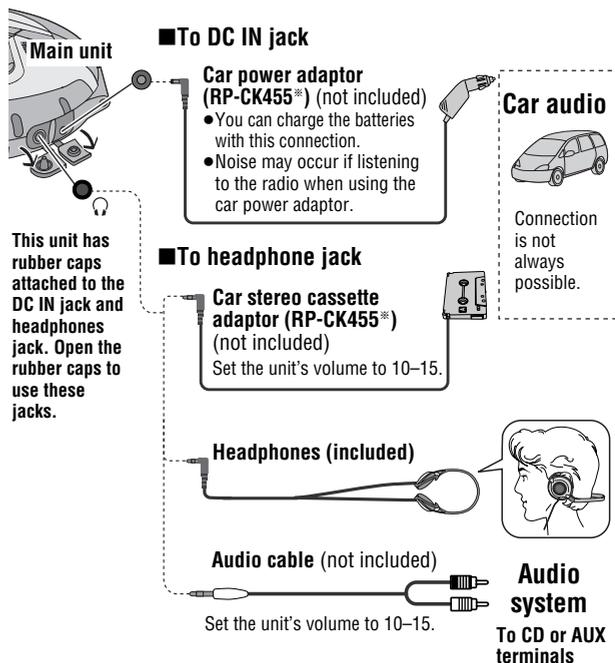
※ The RP-CK455 set contains the car power adaptor and car stereo cassette adaptor. Be sure to use these together for the car audio connection.
