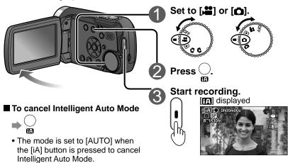
When the camera is pointed at a subject, the mode is determined automatically, and adjustment is made automatically to the optimum settings.
