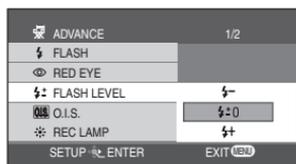
Press the menu button, use the cursor button to select [ ADVANCE ] → [ ± FLASH LEVEL ], then set the desired brightness level. (P27)
