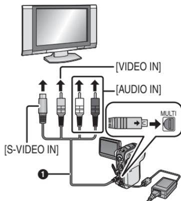
**Open the terminal cover and then connect the multi cable (supplied) to the multi-connector terminal [MULTI] and the TV.**
