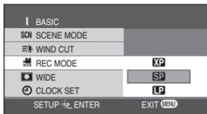
Press the menu button, then use the cursor button to select the desired recording mode by selecting [ ] BASIC]→[ REC MODE]. (P27)
