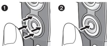
**Press the cursor button up, down, left or right to select items or files ①, and then press the button in the center to enter the selection ②.**
