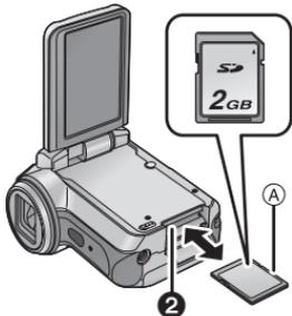
**Insert/remove the SD card into/from the card slot ②.**
