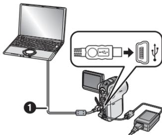
Open this unit's terminal cover, then firmly plug one end of the USB cable **1** (supplied) into the USB terminal and the other end into the terminal on the PC.
