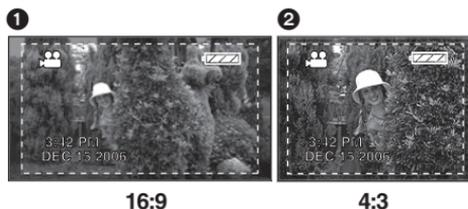
This unit is compatible with wide-screen TVs (16:9) and set to wide mode at the time of purchase. To watch images on normal TVs (4:3), change the wide mode setting before recording (P43) or when playing back the images on the TV screen (P74).
