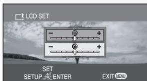
Press the cursor button up or down to select the item to be adjusted. Then, press the cursor button left or right to make the adjustment.
