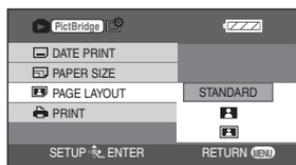
Use the cursor button to select [**PAGE LAYOUT**], then press the cursor button right to enter the layout setting.
