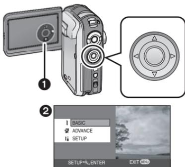
**Press the cursor button to operate the operation icons ① and menu screen ② appearing on the LCD monitor.**
