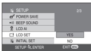
Press the menu button, then use the cursor button to set [ SETUP ] → [ LCD SET ] → [YES]. (P27)
