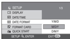
Press the menu button, select [
