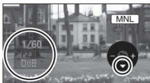
Press the cursor button down several times and select the shutter speed indication (such as 1/60) or iris/gain indication (such as F2.0, 0dB).
