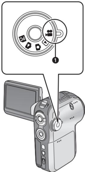
Rotate the mode dial, and set the desired mode pictograph to the position shown in the illustration.
