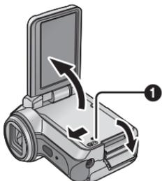
**Open the LCD monitor and then slide the card slot open lever ① to open the card slot cover.**
