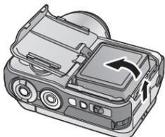
**Remove the battery cover, then remove the battery.**
