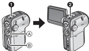
Press the menu button (B), use the cursor button (A) to select [ SETUP ] → [ QUICK START ], and then set the function to [ON]. (P27)
