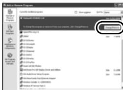
Select the software application to be deleted, then click [Change/Remove] ([Change or Remove] or [Add/Remove]).
