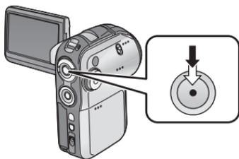
Press the record button halfway (not all the way down) to bring the subject into focus. (In auto focusing mode only)
