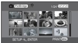
Press the cursor button up or down to select the desired number of prints, then press the button in the center.
