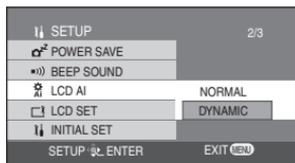
Press the menu button, then use the cursor button to select [ SETUP ] → [ LCD AI ] → [ DYNAMIC ] or [ NORMAL ]. (P27)
