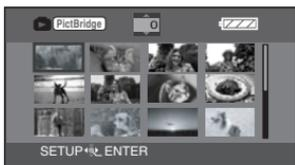
Press the cursor button up, down, left or right to select a scene to be printed, then press the button in the center.
