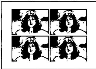
This feature allows you to divide the paper into 4, 9, or 16 mini-frames, and then print the same stored image, reduced in size, in each mini-frame.
