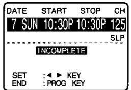
If you push REC on the remote control or the Combination VCR, and a cassette is inserted with no record tab... (see page 29.)
