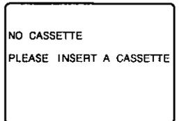
If Combination VCR is not in Stop mode or a cassette with record tab is not inserted two minutes before a Timer Recording is about to begin... (see pages 18, 19.)
