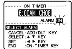
When "ON" is selected, an alarm will gradually increase in volume for one minute or until cancelled by pushing any button on the remote or Combination VCR (including Volume UP/DOWN). When the alarm sound stops, the sound of the mode you selected will ensue.
