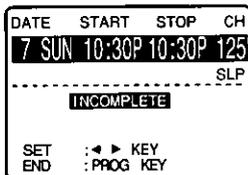
If you push REC on the remote control or the Combination VCR, and a cassette is inserted with no record tab... (see page 41.)
