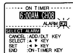
When "ON" is selected, an alarm will gradually increase in volume for one minute or until cancelled by pushing any button on the remote or Combination VCR (including Volume UP/DOWN). When the alarm sound stops, the sound of the mode you selected will ensue.
