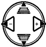
Whenever a menu or program screen is displayed, CHANNEL UP/DOWN and VOLUME UP/DOWN on the remote control function as
