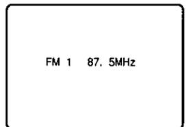
b Push ▲ ▼ to select desired radio station. (Each push changes the frequency by 200 KHz.)
