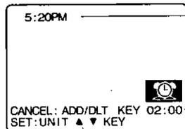
The current time (if clock is set) and time remaining display change positions on the screen every 10 seconds.
