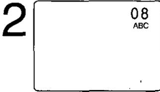
**2** Select a channel. Using CH ▲▼ or NUMBERED keys.
