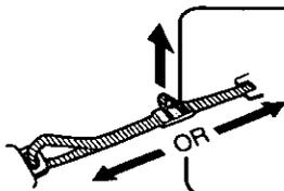
**1** Pull a loop of the strap loose from the buckle.
