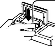
**1** Turn the Tape Wheel on the **VHS** cassette in the direction of the arrow to reduce any slack.
