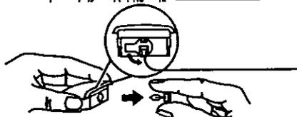
**3** Turn the Bulb Housing counterclockwise 1/4 of a turn and pull free from the Built-in Light unit.
