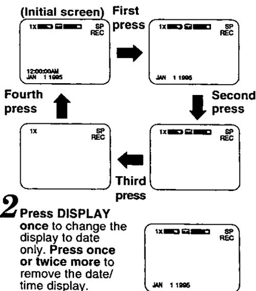
**2** Press DISPLAY once to change the display to date only. Press once or twice more to remove the date/time display.
