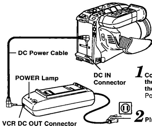
**1** Connect the VCR DC OUT on the AC Adaptor to the DC IN on the Palmcorder with the DC Power Cable (supplied).
