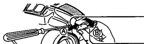
**1** Turn screw counterclockwise and remove.
