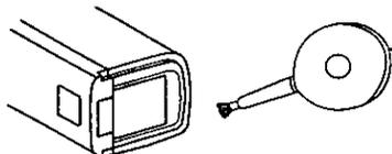
**3** Remove any lint or dust particles with a blower, available at photography stores. Do not touch lenses with fingers. Now, replace the eyepiece.
