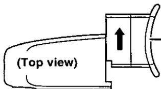
**2** Remove the eyepiece. (Do not twist.)
