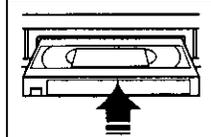
**Insert blank tape with record tab.**
