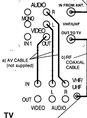
**1** Disconnect antenna or cable from TV and connect to VCR.
