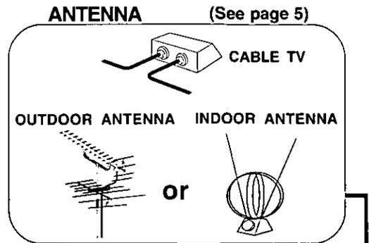
**1** Disconnect antenna or cable from TV and connect to VCR.
