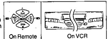
To display menu using VCR buttons, press CH ▲ and CH ▼ together.
