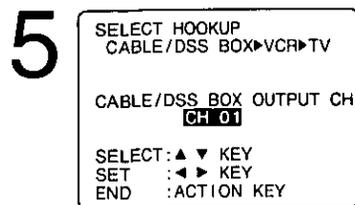
**Select cable box or DSS receiver output channel.**
