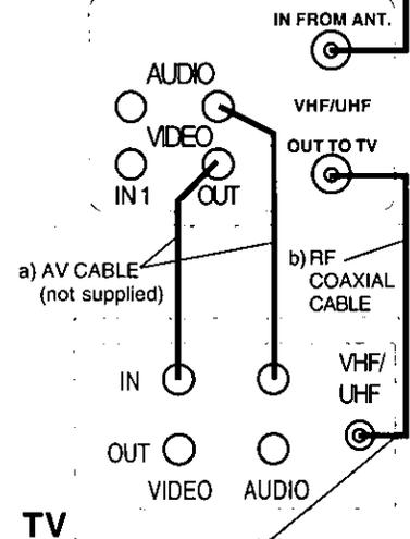
**2** Connect VCR to TV with RF Coaxial Cable.
