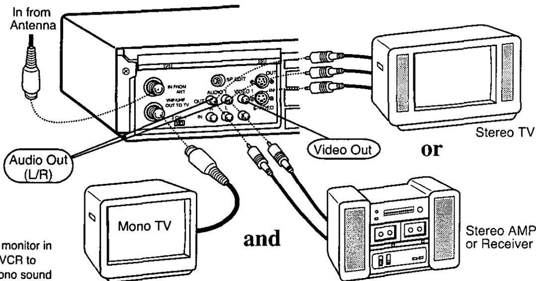
When recording, you may monitor in stereo, by connecting the VCR to either a stereo TV, or a mono sound TV with stereo amp and speakers.
