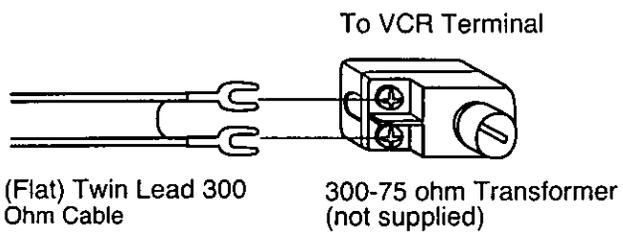
**Case 2: Twin Lead & Coaxial Cables**
