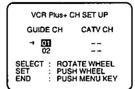
Then, rotate the **Wheel** to change **CATV** or **TV CH** number.
