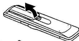
**2** Install three batteries as indicated inside the Battery Compartment.
