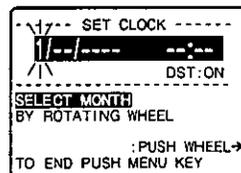
2 Rotate and push the Wheel to select and enter the month, date, year, time and D.S.T. (Daylight Saving Time).
