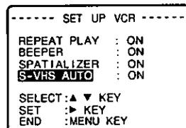
• When you select that "S-VHS AUTO" is "ON," the recording mode is automatically set according to the type of cassette tape used, S-VHS or VHS. When you select that "S-VHS AUTO" is "OFF," recording is done in the normal VHS mode, regardless of the type of cassette tape inserted. Select "OFF" when recording on an S-VHS tape in VHS mode to be played back on a VHS VCR.
