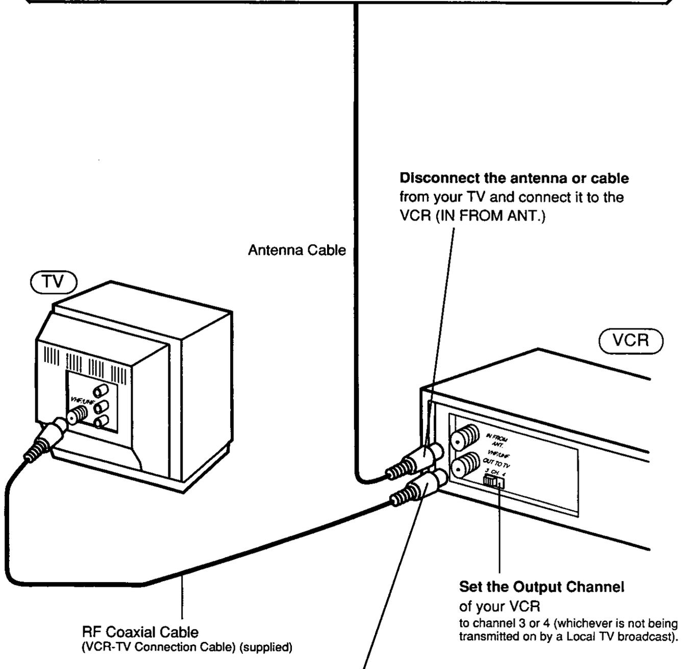
Disconnect the antenna or cable from your TV and connect it to the VCR (IN FROM ANT.)
