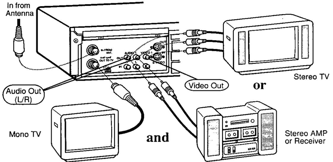
When recording, you may monitor in stereo, by connecting the VCR to either a stereo TV, or a mono sound TV with stereo amp and speakers.
