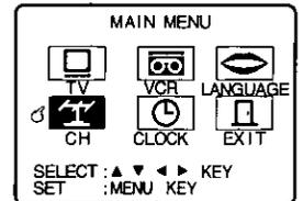
② Push ▲ ▼ ◀ ▶ to select "CH," and then push MENU to display the SET UP CHANNEL screen.
