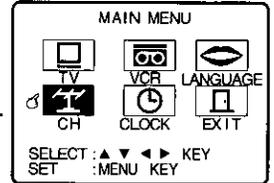
**(b)** Push **▲** **▼** **◀** **▶** to select "CH," and then push MENU to display the SET UP CHANNEL screen.
