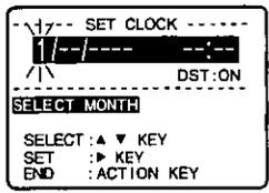
• "DST:ON" automatically adjusts for daylight saving time. (See page 32.)
