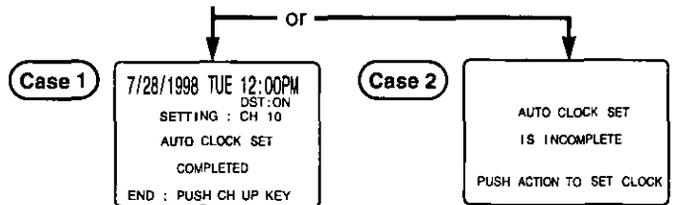
**4** **Case 1** If the displayed time is correct, press **CH ▲** to exit.
