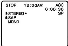
**b** Press **COUNTER RESET** to reset the Time Counter to "0:00:00" at the desired position.
