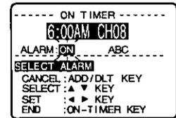
**To Make Corrections,** use **▲▼** and **◀▶** to move back and correct as necessary.
