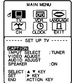
**2** Press **▲▼◀▶** to select "TV," and then press **ACTION** to display the **SET UP TV** screen.
