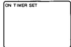
**To cancel,** press **ON-TIMER** to redisplay the screen in step 3. Then, press **ADD/DELETE** to clear the time ("6" is flashing). Now, press **ON-TIMER** to end. "ON TIMER END" appears on-screen for a few seconds.
