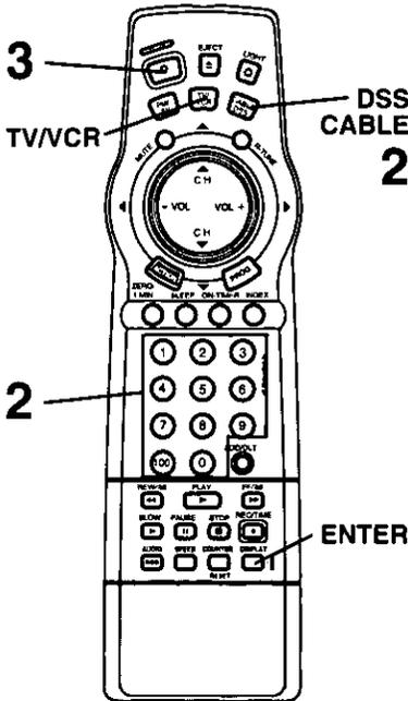
The remote control is designed to control the brands listed. However, it will not operate all DSS Boxes or Cable boxes made by these manufactures. If you get no results, your particular product brand cannot be controlled by this remote.
