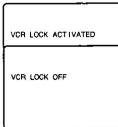
**To Cancel the VCR Lock feature,** with or without a cassette inserted, hold down REC/TIME on the Combination VCR for 7 seconds again during Power On mode.
