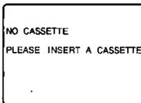
If the Combination VCR is not in Stop mode or a cassette with record tab is not inserted two minutes before a Timer Recording is about to begin... (see pages 18, 19.)
