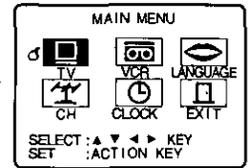
**2** Press **▲▼◀▶** to select "TV," and then press **ACTION** to display the SET UP TV screen.
