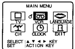
**b** Press **▲▼◀▶** to select "VCR," and then press **ACTION** to display the SET UP VCR screen.
