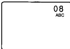
When a function button is pressed (PLAY, FF, etc.), the Combination VCR mode will be displayed.
