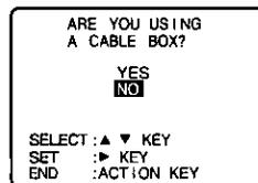
Select **YES** if all channels are received via the cable box (connection "A" at left). Then, go to step 5.
