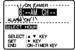
**2** Press **▲▼** to select and **▶** to fix the On-Timer time and also to choose the On-Timer mode (TV, PLAY, or FM radio). See the **▲▼** selection order shown below.
