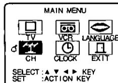
**2** Press **▲▼◀▶** to select "CH," and then press **ACTION** to display the SET UP CHANNEL screen.
