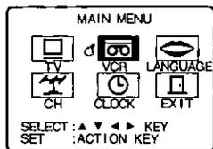
**2** Press **▲▼◀▶** to select "VCR," and then press **ACTION** to display the SET UP VCR screen.
