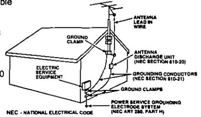
provides information with respect to proper grounding of the mast and supporting structure, grounding of the lead-in wire to an antenna discharge unit, size of grounding conductors, location of antenna discharge unit, connection to grounding electrodes and requirements for the grounding electrode.
