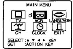
**2** Press **▲▼◀▶** to select "VCR," and then press **ACTION** to display the SET UP VCR screen.
