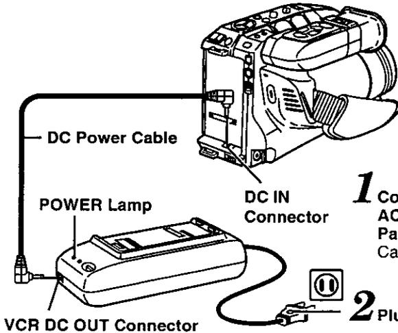
**1** Connect VCR DC OUT on the AC Adaptor to DC IN on the Palmcorder with the DC Power Cable (supplied).
