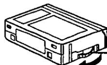
**1** Turn the Tape Wheel on the **VHS** cassette in the direction of the arrow to take up any slack.
