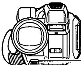
**1** Press **MANUAL FOCUS** so that "MF" (Manual Focus) appears in the EVF.
