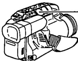
**4** Press the "W" side of the **POWER ZOOM** switch to frame the picture as desired.
