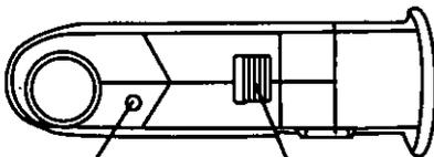
**\*Note:** This control has been set at the factory. It is not necessary to adjust this control under normal circumstances. But, should it become necessary, be careful to make the adjustment with a small, slender screwdriver so as not to damage the miniature control.
