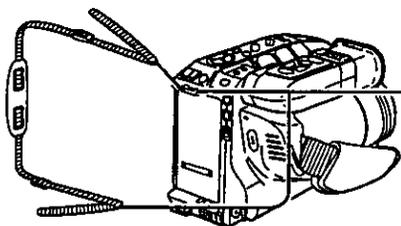
**2** Thread the strap ends through the Strap Attachment Rings.
