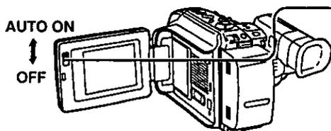
**2** Set the LCD-POWER switch to AUTO ON. The LCD monitor will then turn on/off according to the Palmcorder's POWER switch setting.
