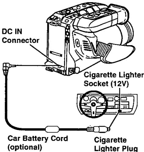
**1** Connect a PV-C16 Car Battery Cord (optional) to DC IN on the Palmcorder.
