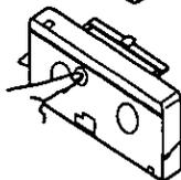
**2** Hold the PlayPak securely in one hand. Using your finger, reach through the hole in the bottom of the PlayPak Adaptor and push the tape out the top.
