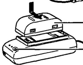
**2** Place the Battery into the AC Adaptor.
