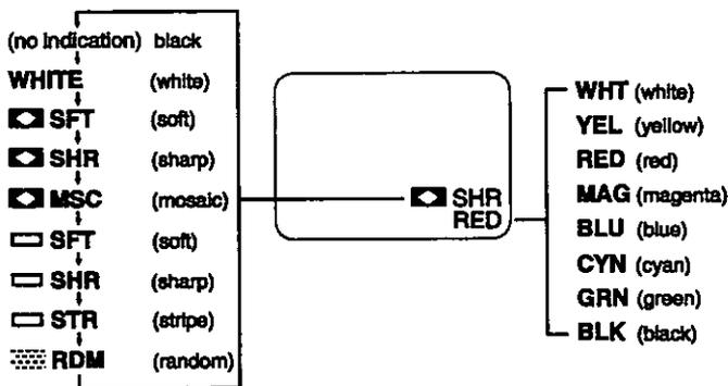
■ Create more effects: You can stop the fade at any time by pressing the **MODE SEL** button (other than BLACK, WHITE, and RANDOM modes). Pressing the **FADE** button will continue the fade. Pressing the **MODE SEL** button will cancel the fade.
