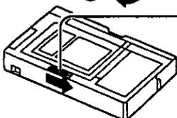
**2** Slide the **RELEASE** button in the direction of the arrow to open the PlayPak door.
