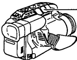
**3** Turn the **MANUAL FOCUS** control until the picture is in focus.
