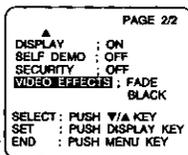
**3** Press DISPLAY for VIDEO EFFECTS menu. Press DOWN ▼ to select DIGITAL FADE.
