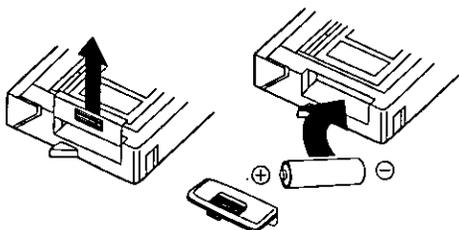
Remove Battery lid and insert AA battery.
