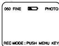
**4** Press **MENU** for **REC Mode**. Press **UP ▲** or **DOWN ▼** to select **NORMAL** or **FINE** (page 75). Then, press **DISPLAY** to set.
