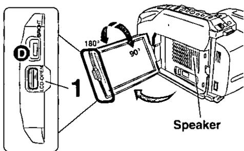
**1** Press **LCD-OPEN** and swing LCD monitor fully open.
