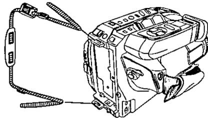
**4** Thread strap ends through Strap Rings on Camcorder.
