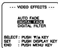
**4** Press DISPLAY for DIGITAL FADE menu. Press UP ▲ or DOWN ▼ to select TYPE. Press DISPLAY for TYPE menu. Press UP ▲ or DOWN ▼ to select from 7 types.
