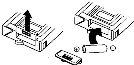
Remove Battery lid and insert AA battery.
