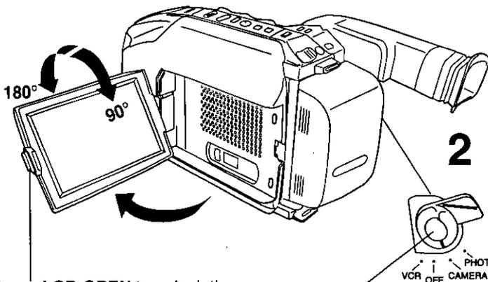
1 Press LCD-OPEN to unlock the LCD monitor. Swing it fully open and adjust the angle.
