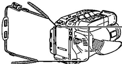
**4** Thread the strap ends through the Strap Attachment Rings.
