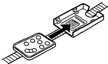
This holder (supplied) can be attached to the shoulder strap (see page 21). When the Remote is not in use, slide it into the holder as shown.
