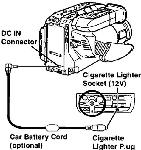
**1** Connect a PV-C16 Car Battery Cord (optional) to DC IN on the Camcorder.
