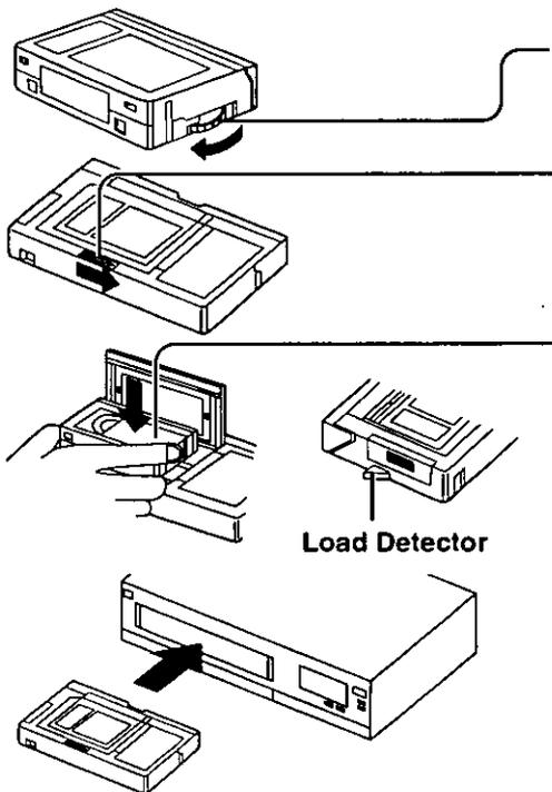
**1** Turn the Tape Wheel on the **VHS** cassette in the direction of the arrow to take up any slack.
