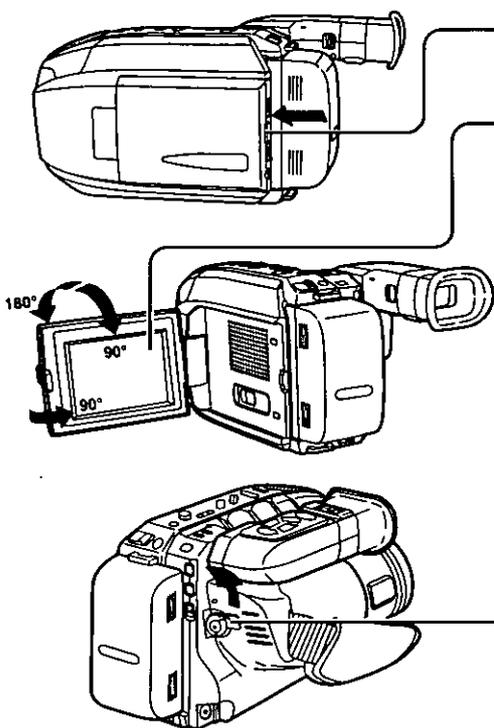
**1** Press the LCD-OPEN button to unlock the LCD monitor.
