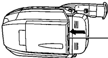
**1** Press the LCD-OPEN button to unlock the LCD monitor and swing it open.
