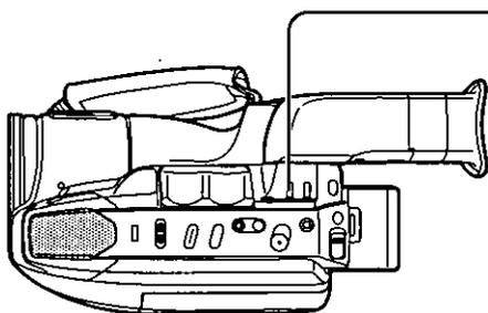
**1** Press HIGH SPEED SHUTTER while recording.
