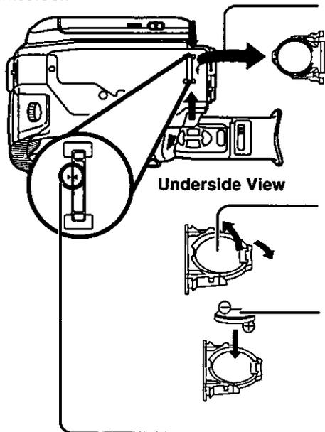
**1** While pinching the stopper tabs, pull the Battery Tray out of the Battery Compartment.
