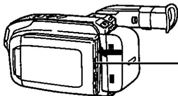
**1** Press the **LCD-OPEN** button to unlock the LCD monitor and swing open.
