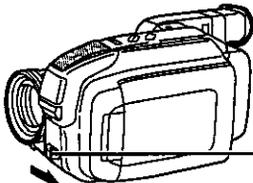
**5** Set POWER switch to CAMERA. Built-In Lens Cover opens and POWER Lamp lights.
