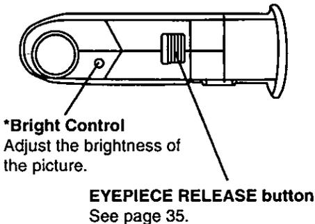
**\*Note:** This control has been set at the factory. It is not necessary to adjust this control under normal circumstances. But, should it become necessary, be careful to make the adjustment with a small, slender screwdriver so as not to damage the miniature control.
