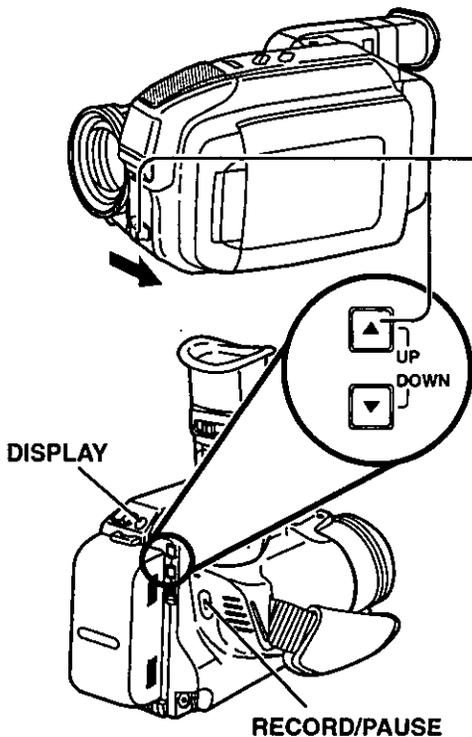
**1** Continue holding down the UP ▲ button before and after turning the POWER switch to CAMERA until the STAND-BY RELEASE menu screen is displayed.
