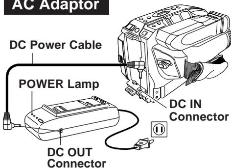
**1** Connect AC Adaptor DC OUT to Camcorder DC IN with supplied DC Power Cable.
