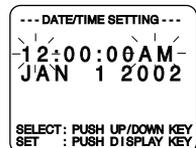
Press or hold down **UP** or **DOWN** to select hour, then press **DISPLAY** to fix.
