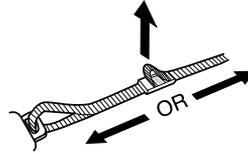
Pull a loop of strap from buckle, then pull strap tight to shorten or lengthen.
