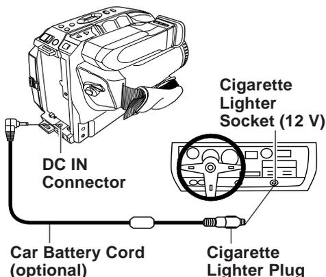
**1** Connect PV-C16 Car Battery Cord (optional) to Camcorder DC IN.
