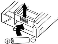
Remove Battery lid and insert AA battery.
