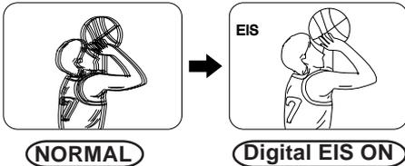
**1** Press **EIS** to display "EIS" in the EVF or LCD monitor.
