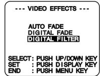
**3** Press **DISPLAY** for DIGITAL FILTER menu. Press **UP** or **DOWN** to select from 5 colors.
