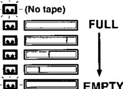
• Tape remaining indicator operates a few seconds after tape starts moving.
