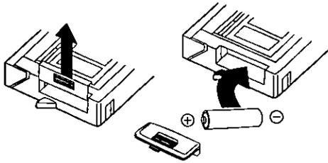
Remove Battery lid and insert AA battery.
