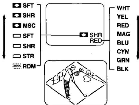
■ For more effects, stop fade in or fade out at any time (except RANDOM mode) by pressing FADE. Then, press FADE to resume fade.
