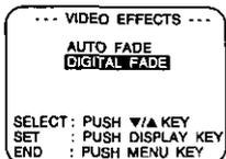
**3** Press **DISPLAY** for DIGITAL FADE menu. Press **UP ▲** or **DOWN ▼** to select **TYPE**. Press **DISPLAY** for TYPE menu. Press **UP ▲** or **DOWN ▼** to select from 7 types.
