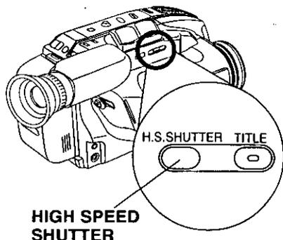
**1** Press **HIGH SPEED SHUTTER** while recording.
