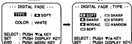
**4** Press **DISPLAY** for DIGITAL FADE menu. Press **DOWN ▼** to select **COLOR**. Press **DISPLAY** for COLOR menu. Press **UP ▲** or **DOWN ▼** to select from 8 colors.
