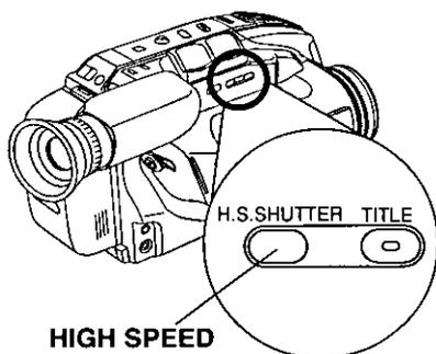
**1** Press **HIGH SPEED SHUTTER** while recording.
