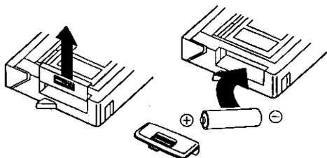
Remove Battery lid and insert AA battery.
