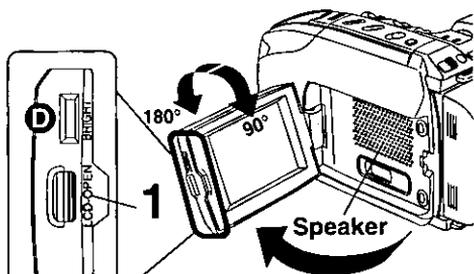
**1** Press **LCD-OPEN** and swing LCD monitor fully open.
