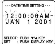
Press or hold down **UP ▲** or **DOWN ▼** to select hour, then press **DISPLAY** to fix.
