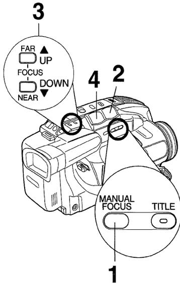
**1** Press **MANUAL FOCUS** so "MF" (Manual Focus) appears in EVF or LCD monitor.
