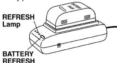
To use battery refresh, insert Battery on AC Adaptor (see steps 1~2 above), then press **BATTERY REFRESH**.
