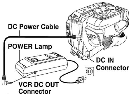
**1** Connect AC Adaptor VCR DC OUT to Camcorder DC IN with supplied DC Power Cable.
