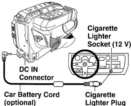
**1** Connect PV-C16 Car Battery Cord (optional) to Camcorder DC IN.
