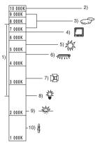
Outside of the effective range of Automatic White Balance Adjustment, the image will become reddish or bluish. Even within the effective range of Automatic White Balance Adjustment, the Automatic White Balance Adjustment may not function properly if there is more than one light source. In this case, adjust the White Balance.
