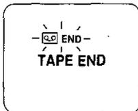
When the tape is about to end in REC mode, "REC" will flash and "TAPE END" will appear for 5 seconds.
