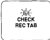
If the Palmcorder is in CAMERA mode with the cassette sliding record tab opened, "REC" will flash and "CHECK REC TAB" will appear for 5 seconds. Recording will not start.
