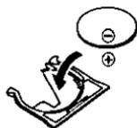
**2** Insert the battery into the Battery Tray with the ⊖ mark facing up. Do not reverse the polarity.
