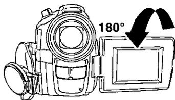
Rotate the LCD monitor 180 degrees so that it faces in the same direction as the lens while in the CAMERA mode to record yourself.
