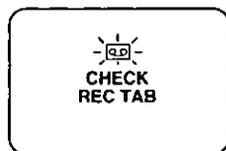
If the Palmcorder is in CAMERA mode with the cassette sliding record tab opened, "REC" will flash and "CHECK REC TAB" will appear for 5 seconds. Recording will not start.
