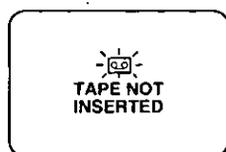
If the Palmcorder is in CAMERA mode without a cassette inserted, "REC" will flash and "TAPE NOT INSERTED" will appear for 5 seconds. Recording will not start.
