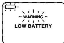
When a battery recharge is necessary, "WARNING" will flash, "LOW BATTERY" will appear, and the Palmcorder will automatically turn OFF in 15 seconds (page 26).
