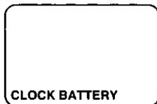
When the built-in lithium clock battery is discharged, "CLOCK BATTERY" will appear. To re-charge the lithium clock battery, connect the AC Adaptor to the Palmcorder. Recharging takes approx. 4 hours. Reset the clock after charging.
