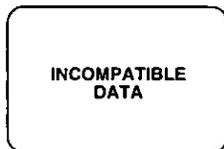
If you play a tape recorded in a format other than NTSC or you try to copy a copy-protected tape, "INCOMPATIBLE DATA" will continuously appear. This message also appears if REC is pressed when DV is input and the copy of copyrighted information is prohibited.
