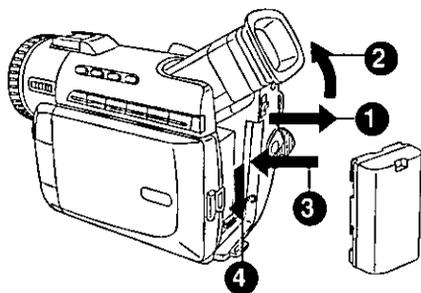
**1** Slide the Viewfinder backward to its fully extended position and then tilt it upward. (For model PV-DV200, Tilt Viewfinder upward.)
