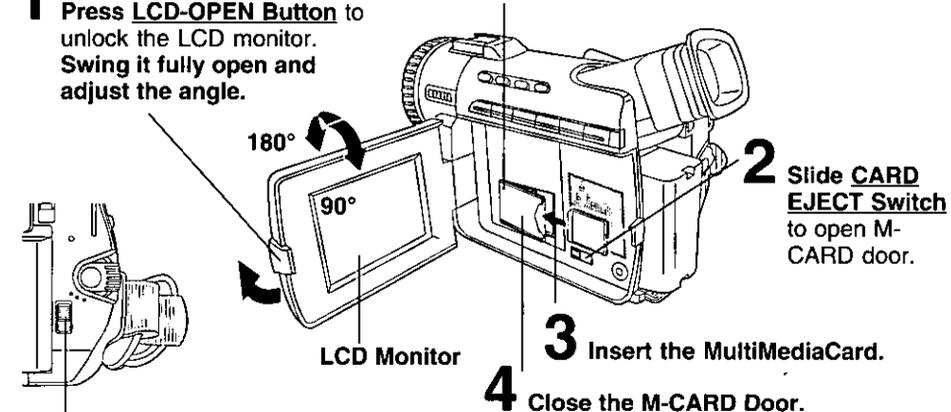
When using a MultiMediaCard, you must set **TAPE/M-CARD Switch** to M-CARD.
