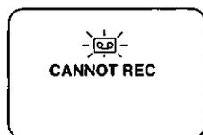
When Audio dub is performed and the sliding record tab is open, or a blank portion of tape is detected, "REC" will flash and "CANNOT REC" will appear for 5 seconds.
