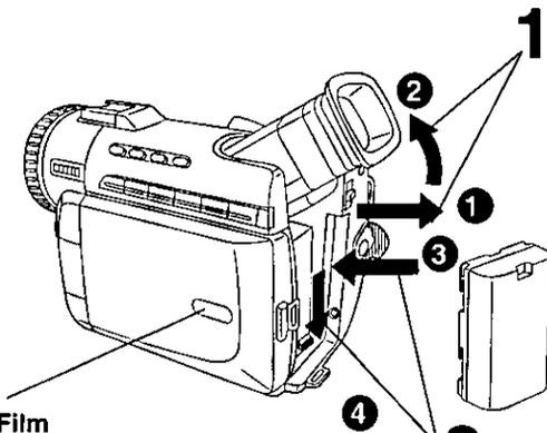
**1** Slide the Viewfinder **backward** to its fully expanded position and then tilt it upward. (For model PV-DV200, Tilt Viewfinder upward.)
