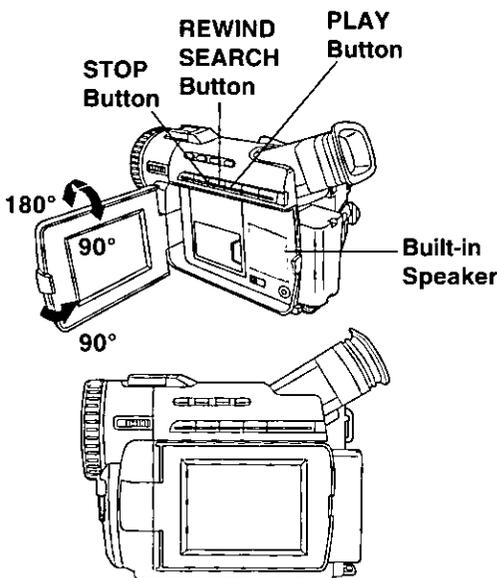
You can place the Palmcorder on a table, etc. for viewing. Rotate the LCD Monitor 180° and swing it up against the Palmcorder body as shown.
