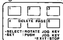
**3** Rotate and press **JOG KEY** to select and set the image to be deleted.
