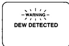
If excessive moisture condenses in the unit, "WARNING" will flash, "DEW DETECTED" will appear, and the Palmcorder will automatically turn OFF in 15 seconds. In this case, wait until the indicator no longer flashes when your Palmcorder is turned on again.
