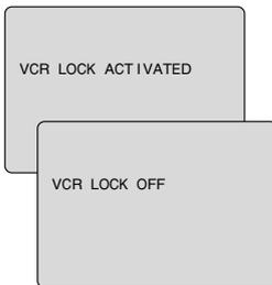
In stop mode, **hold down REC** on the unit without a cassette inserted for 7 seconds to turn "ON." Please ignore NO CASSETTE warning.
