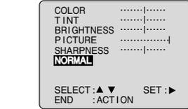
**To Reset Picture Controls,** press **▲▼** and **▶** to select and set "NORMAL". All controls return to their factory settings.
