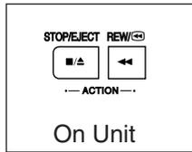
You can operate the menu screen using unit buttons. To display the menu, press STOP/EJECT and REW together with no tape inserted. To exit the menu, repeat above with or without tape inserted until normal screen appears.
