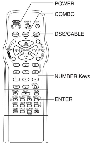
**\*Important:** If a remote control button does not work when pressed, press the COMBO button on the remote and try the button again.
