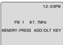
**1) Press CH ▲▼** to select the desired radio station. (Each press changes frequency 200 kHz.)
