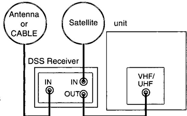
NOTE: The DSS receiver must be turned off to view programs from a cable box or antenna. See the DSS manual for details.
