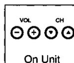
Whenever the menu or program screen is displayed, CHANNEL UP/DOWN function as ▲▼ and VOLUME UP/DOWN function as ◀▶ only.
