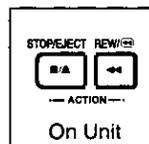
You can operate the menu screen using unit buttons. To display the menu, press STOP/EJECT and REW together with no tape inserted.
