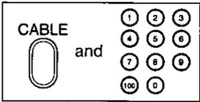
Hold down CABLE and enter code with NUMBERED keys.
