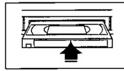
Insert blank tape with record tab.
