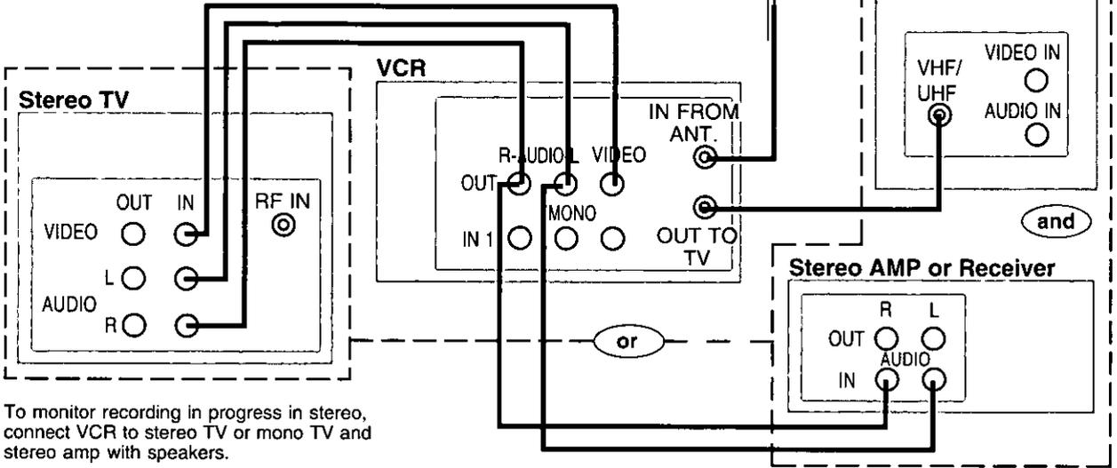
To monitor recording in progress in stereo, connect VCR to stereo TV or mono TV and stereo amp with speakers.
