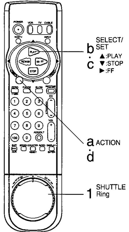
\*Important: If the remote control POWER, ACTION, CH▲/▼, INDEX, NUMBERED keys, INPUT, ADD/HLT, or DISPLAY button does not work when pressed, press the VCR button on the remote and try the button again.
