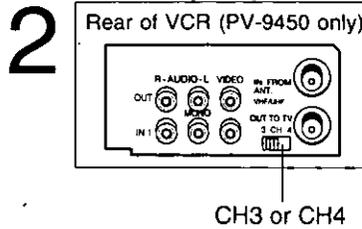
**2** Tune to VCR output channel. Tune TV to CH3 or CH4. (Same as back of VCR)
