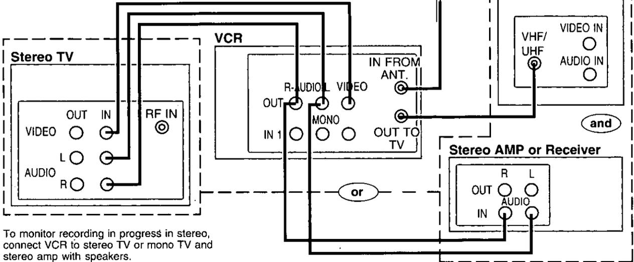
To monitor recording in progress in stereo, connect VCR to stereo TV or mono TV and stereo amp with speakers.
